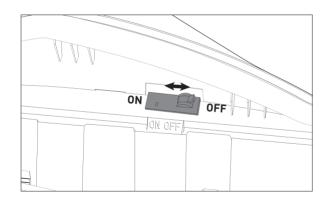
TIPS: In order to protect your safety, please turn off the circuit protector switch when cleaning, storing the vehicle for a long time, or removing the battery.
